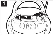
Press the POWER button **①** to the in position and slide the Function switch **②** to the CD position. Insert a CD as described in the TO INSERT A CD section on page 6.
